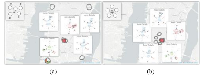
Figure 6: Given positions of AOIs selected by users, our system can adaptively put detail views around them. Sub-figures in the top-left corner show thumbnails of the layout. Grey nodes and white nodes denote AOIs and details respectively. Five AOIs (a) far from each other. (b) close to each other.
