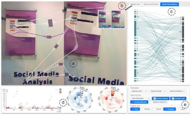
Figure 2: VisFM system interface. (a) A matching view shows both bundled matching data and segments of images; (b) a feature view presents the feature data through a heat map and a zoom-in/zoom-out interactive mode; (c) a group view shows the matching relationships of feature groups between two images; (d) a feature scatterplot view and a circular heat view provide additional explorations of the features and (e) an option panel supports parameter setting and interaction mode switching.
